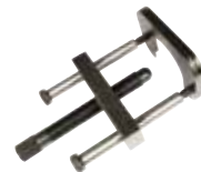
Crank gear puller When using this tool heat should still be applied to the gears. Not for diesel engines.
