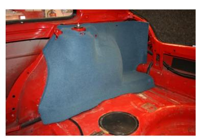
To fit this wheel arch cover you will need to take several parts of the trim apart. Initially you will need to remove the rear seats, the rear quarter panel and the two panels adjacent to the rear parcel shelf. The easy part is to just remove the old wheel arch and replace it with our new one. We would suggest you apply spray adhesive to the lower areas of the carpet to hold them in place.
