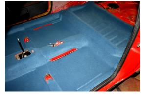
distorted in the moulding process. If you are a purist, you may want to cut some of this area away to make it look like the original Factory shape. The areas around the seat slides are already cut away, but make sure the carpet is tucked behind these runners so as not to interfere with the seat movement. We have not cut holes for the rear seat base – you will find on the back of the carpet some dimples in the moulding which will indicate where these holes are located.
