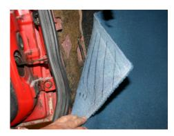
secure the carpet in place. Note - where we have drawn lines on the back of the carpet-glue in this area. This will apply to the passenger side as well.
