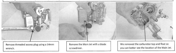
Main Jet Installation and Removal Tip: After loosening the main jet with a screw driver, use a wooden tooth pick to remove. Using the same toothpick, you can start the replacement jet, remove the toothpick and tighten with the screwdriver.
