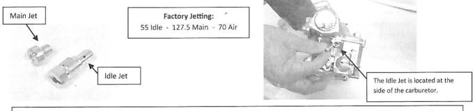
The Main Jet is located in the float bowl. Remove threaded access plug (14mm), then remove jet. You can remove and replace the Main Jet without removing the carburetor top. However, removing the carburetor top and float allows you to see the Main Jet – making it easier to re-install the jet.
