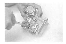
10. If you have followed this procedure and the engine will not idle, most likely the cause is a vacuum leak. Start from the top and repeat.
