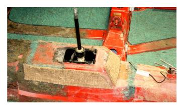
**Stage Three** – You will find two main tunnel felts. Place the large piece over the tunnel as shown and glue in place. Now glue the second felt on top of the first one.
