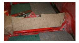
**Stage Six** – The two longer parts can now be glued over the cables as shown here.
