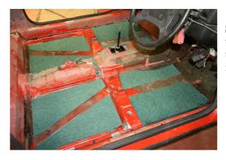
**Stage Two** – These three pieces need to be glued to the top rear of the tunnel by the gear lever. You will see there is a recess in the metal and these pieces will fill that gap.
