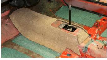
**Stage Four** – Place and glue the last tunnel piece in place as shown here. Join all the edges for a smooth finish.
