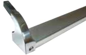
Easier access to your side door with this extruded aluminium step with polished cast ends. Fixes to jacking points and is supplied with stainless steel hardware. Will not fit Brazilian Bus. Fits all years
