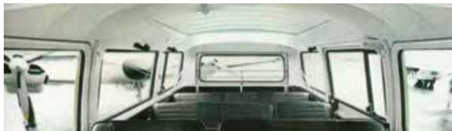
Headliners, available in vinyl crush, vinyl perforated & cloth. We indicate the correct number of tensioning bows for each item, these are available separately if required, see below. NOTE. TMI themselves recommend the use of an experienced fitter for all full length headliners.
