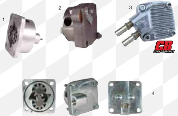
Please check which type of camshaft you are using before you purchase your oil pump. Camshafts are either "early" 3 rivet/bolt (>1971) or "late" 4 rivet/bolt (1972). This affects the depth of the oil pump. All performance camshafts are of the earlier style.
